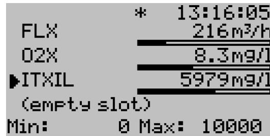
The tag name (max 10 characters) can be changed in the sensor menu, default is the type of sensor.
