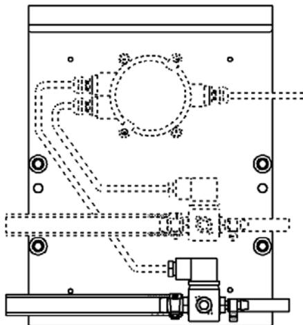
Mounting plate (non US version) with two solenoid valves P/N 11705516B, and a connection box P/N 11505748.
