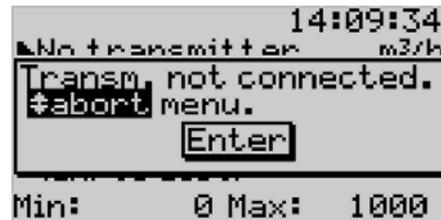
To access the menu of a sensor that is not connected, change the highlighted text from “abort” to “show” using the arrows and press **ENTER**.
