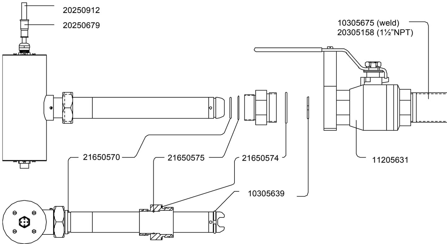
Nipple 10305675 is to be cut to make the bottom of the measure gap be at least 5 mm (¼") from the pipe wall.
