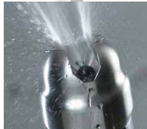
The automatic flushing device has no moving parts and ensures minimal maintenance and enhanced reliability. The flushing nozzle uses water or compressed air.
