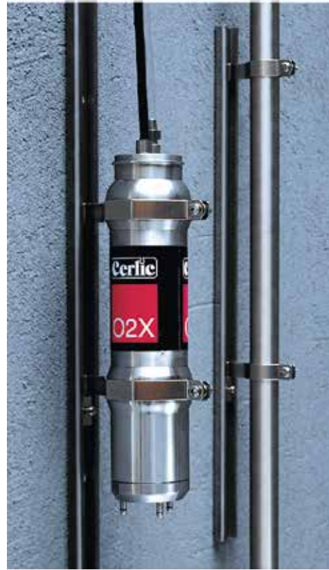
SS Slide rail assembly for easy installation and servicing. Available in two sizes 20 mm Ø for pHX, ReX and FLX and 66 mm Ø for O2X and ITX sensors. The rail has field adjustable stop. It's easy to install and to inspect sensors for cleaning and calibration.
